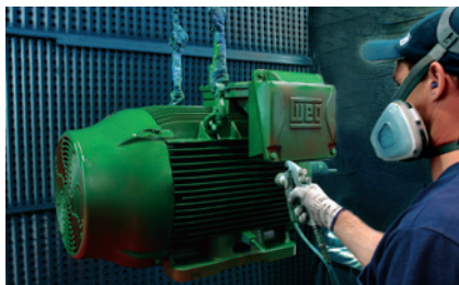
Figure 9 - WEG internal painting plan
